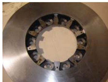
Figure 4. Part Number 10009970. Note thinner mounting flange.
