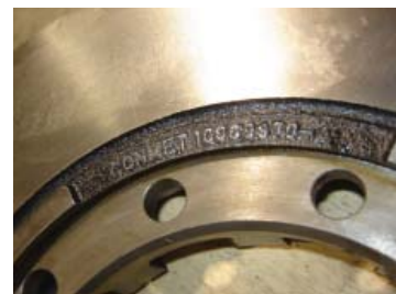
Figure 2. Part Number 10009970 is cast on the face of the rotor above the mounting holes.
