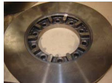
Figure 5. Part Number 10016195. Note thicker mounting flange.
