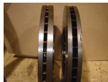
Figure 3. The 10016195 rotor on the left has one braking plate thicker than the other. Also note the difference in the thickness of the web between the braking surfaces.
