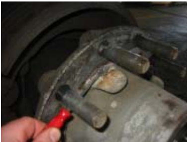
Rust and corrosion build-up.
